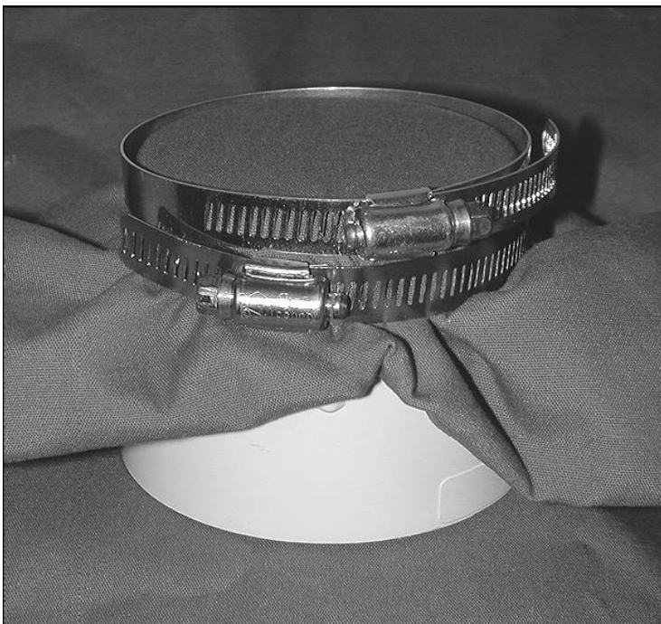
Figure 4. Clamps and “frame” (3” flange) showing how these are assembled to carry out a fabric test.
